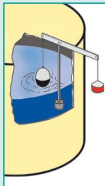
The weighted float and indicator are connected to the counter-weight by separate cords, each cord running over a pair of pulleys.
