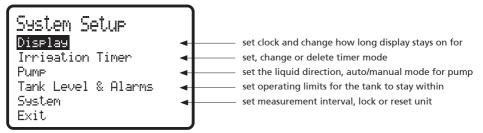
Note: Changes made in Display Unit are instantly transmitted to the Control Unit. However the Tank Unit will only update at the next scheduled reading interval. To force an update remove the Tank Unit lid and press the reset button.
