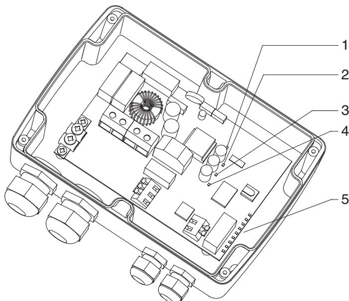
Fig. 14 Position of the LEDs inside the CU 301
