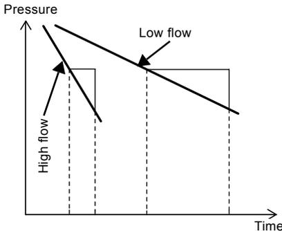
**Fig. 3** Pressure changes in relation to flow
