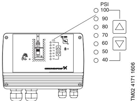
Fig. 10 Pressure setting and indication
