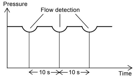
**Fig. 4** Flow detection every 10 seconds during operation
