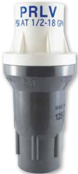
The **Pressure Regulating Limit Valve™** is designed to handle flows from 0.5 to 18 gpm (114 to 4088 L/hr). It is used in place of standard pressure regulators to limit static (no flow) water pressure when a shut-off valve is used downstream from a regulation point. This limits downstream pressure and protects downstream components.
