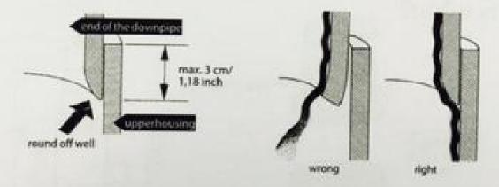
Important: Especially at the uppermost cut the inner edge of the downpipe's end must be rounded well with a file so the water can flow unobstructed onto the inner side of the upper housing. If necessary the end of the downpipe must be widened by flanging.
