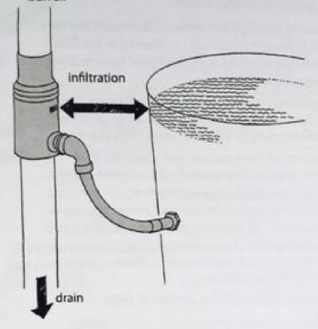
Integrated security overflow: the overflow-mark on the GRS-housing (= WISY-sign) has to be levelled on the desired height of the maximum water level of the barrel. Thus the excess rainwater will automatically be diverted to the infiltration or drain.
