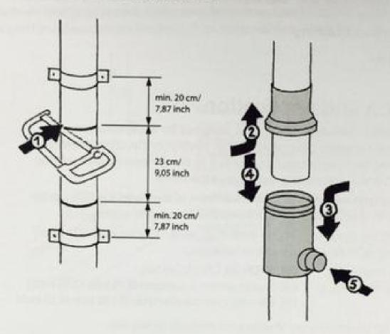
☑ In the desired installation height of the GRS cut out a section of 23 cm
